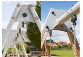
The A-Frame is designed with hot dip galvanised ø100mm crossbar with large steel end plates for strong fixation of the two post options: Hot dip galvanised ø70mm steel. Impregnated pine wood with hot dip galvanised steel footings.
